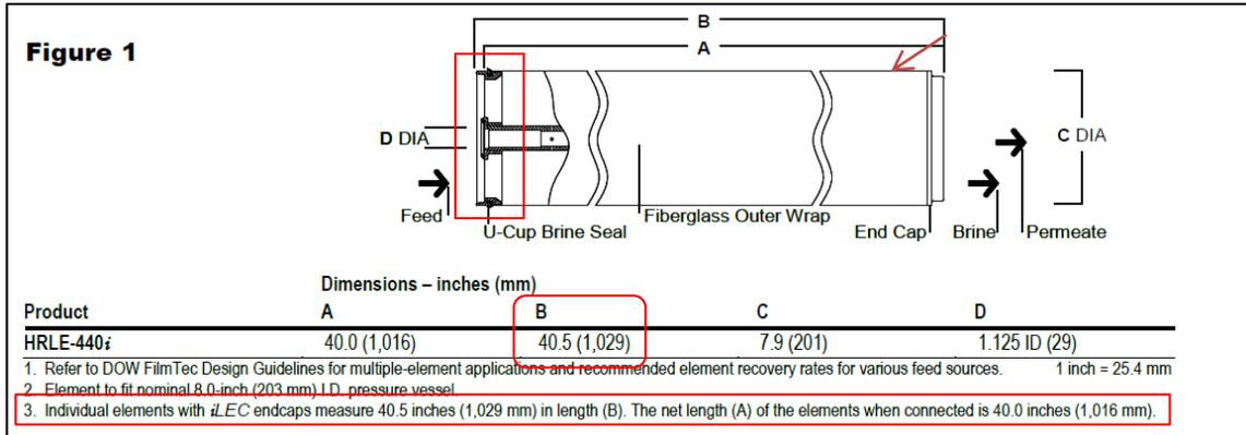
If we bear in mind that in the point 3 of the previous figure its indicated that, once all the elements are interconnected, each membrane fits in its following of the added measure 0,5" which this membrane have, the last membrane would sum up the total length of 40,5".
