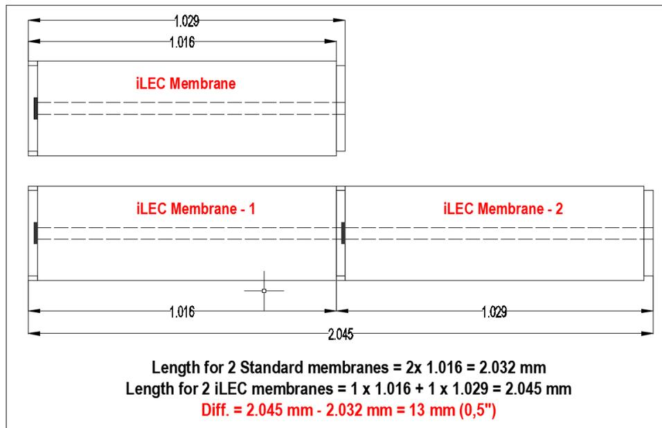
This fact will imply that in order to close the End caps of the pressure vessels, two types of End caps should necessarily be supplied:
