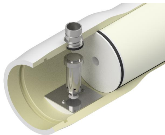
Picture 4.9.5.2 Be sure that the manual pusher is aligned with the side port axis.
