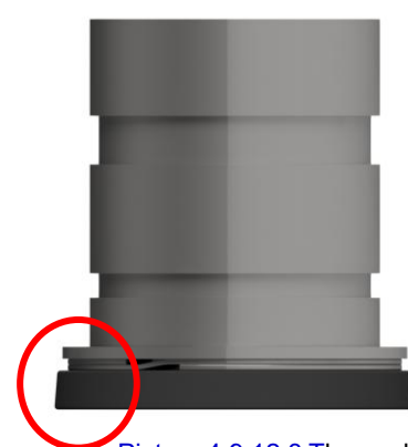
Picture 4.9.12.3 The seal is trapezoidal in shape. The larger diameter should be on the bottom.
