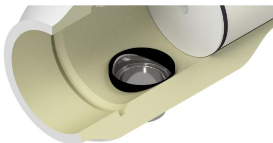
Picture 4.10.14.1. Side port Assembly before remove the excess of rubber.
