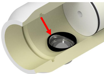
Picture 4.10.16.1. To start the cut, use this point or its symmetrical.
