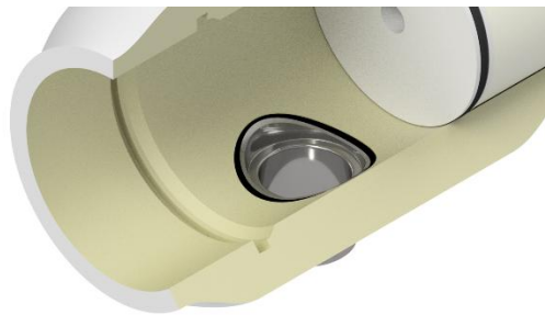
Picture 4.10.14.2. Side port Assembly after remove the excess of rubber.
