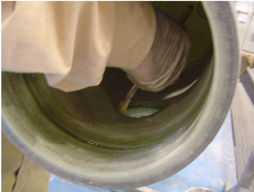
Mix hardener-epoxy application using a brush
